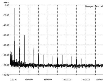
Graph 2: Total harmonic distortion (THD) at 1kHz at an output of 1-watt into a 4-ohm non-inductive load, referenced to 0dB. [Audio Analogue Maestro Integrated Amplifier]
