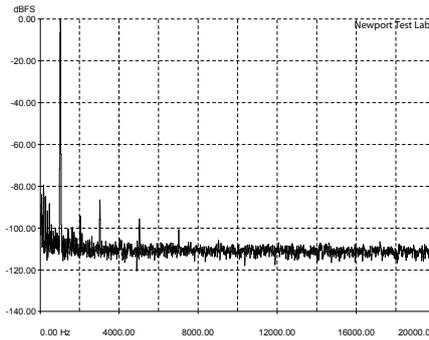
Graph 1: Total harmonic distortion (THD) at 1kHz at an output of 1-watt into an 8-ohm non-inductive load, referenced to 0dB. [Audio Analogue Maestro Integrated Amplifier]
