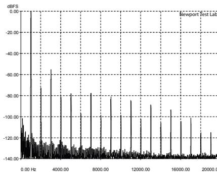
Graph 3: Total harmonic distortion (THD) at 1kHz at an output of 150-watts into an 8-ohm non-inductive load, referenced to 0dB. [Audio Analogue Maestro Integrated Amplifier]
